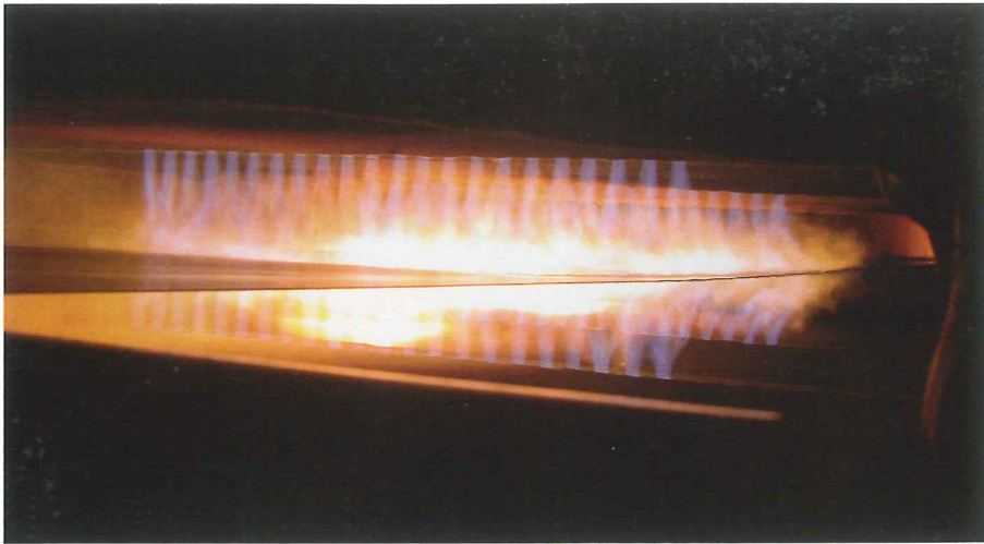
Fig. 6: REBOX DFI at ThyssenKrupp Steel at Finnentrop: oxyfuel flames are heating directly onto the moving strip
