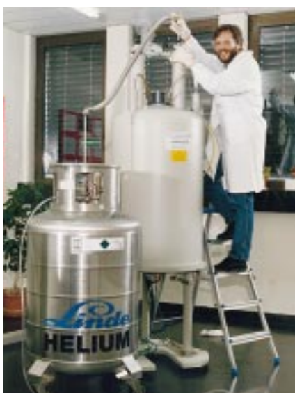
Filling an NMR spectrometer with liquid helium (LHe). The spectrometer is being used for the structural analysis of chemical compounds.
