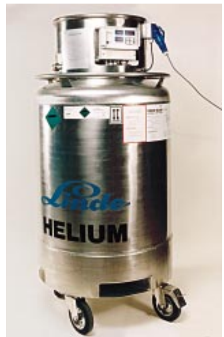
New LHe container with submersible withdrawal pipe, level meter and electronic internal pressurization system.
